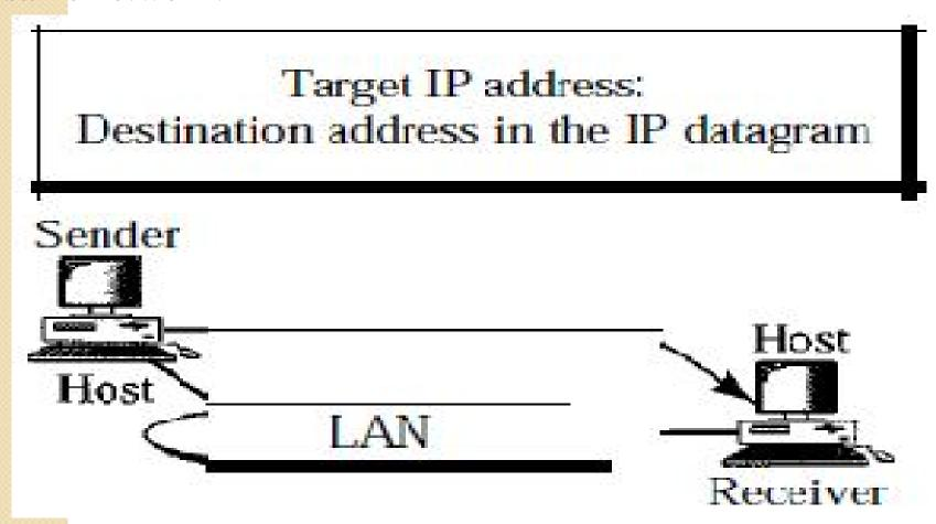
In this case, the logical address that must be mapped to a physical address is the destination IP address in the datagram header.
