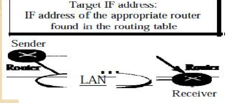
The sender is a router that has received a datagram destined for a host on another network. It checks its routing table and finds the IP address of the next router. The IP address of the next router becomes the logical address that must be mapped to a physical address
